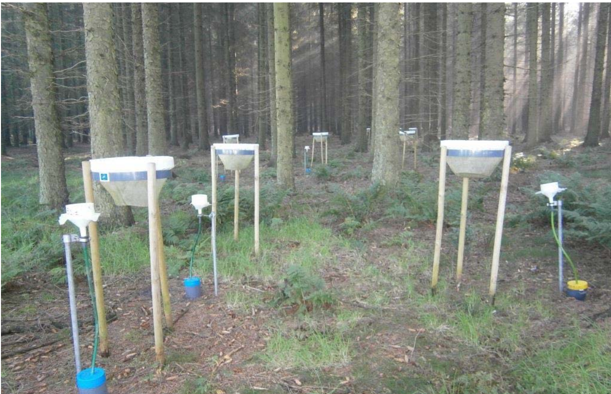
Sampling of litterfall and throughfall in forest edges were performed to monitor the input of C and N to the soil. Here in Sitka spruce at Sønder Omme, Denmark in 2011. (Photo: Shimon Ginzburg)
